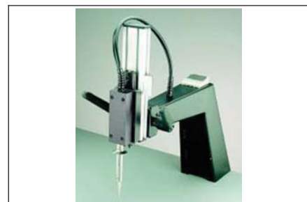
Figure 8 Bond the new land using a Bonding System.
